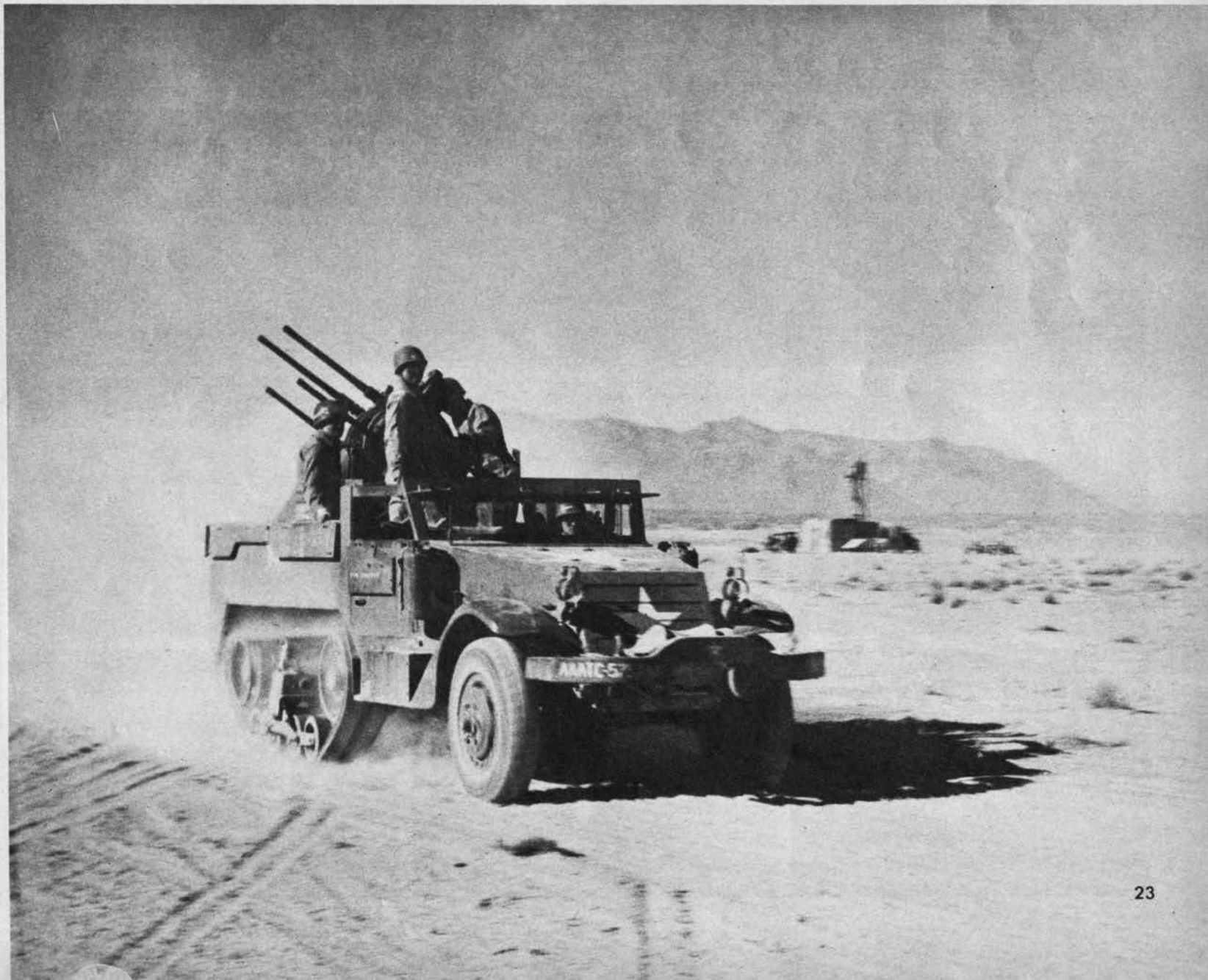
U. S. half-track also acts as SP mount for AA artillery. The M-16 illustrated here has four coaxial .50-cal. machine guns on a rotating mount. Top portions of the half-track's vertical sides fold down on
